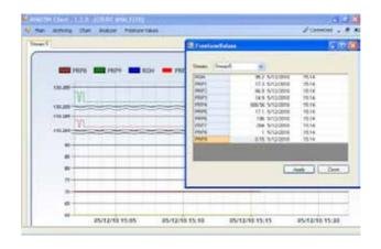
ANACON is a full-distributed analyzer management and control system that has been developed to provide more efficient tools for maintenance, calibration and validation of analyzer systems. It is designed for connection with remote systems using communication links such as TCP/IP or RS-485. ANACON is compatible with the Microsoft Windows platform.
